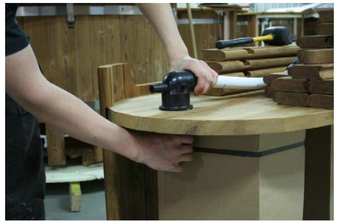
Use the included tool to screw the drainage valve in place.
