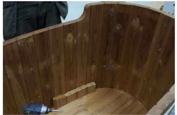
Fasten all the pieces in the side as the picture shows. **NOTE!** The first and last piece are not identical, see picture. Repeat the procedure for the other side.
