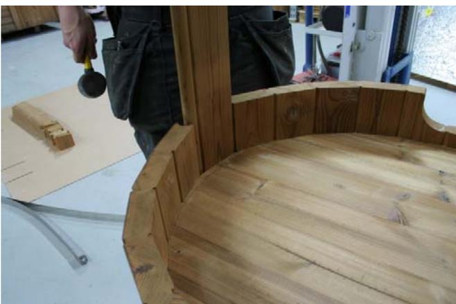
Insert the last stave from above and tap it into its notch with the help of a rubber mallet. All staves are now assembled.
