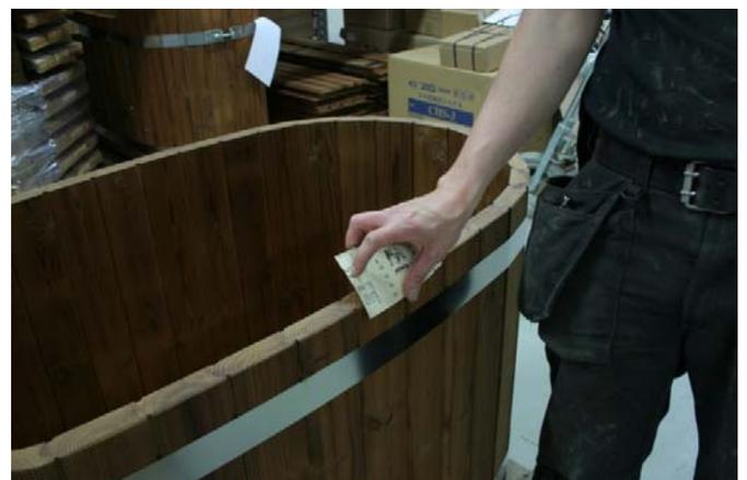
Also bevel the upper edges of the tub.
