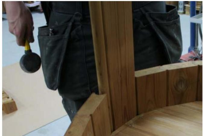
Insert the last stave from above and knock it in place using a rubber mallet. All staves are now assembled.
