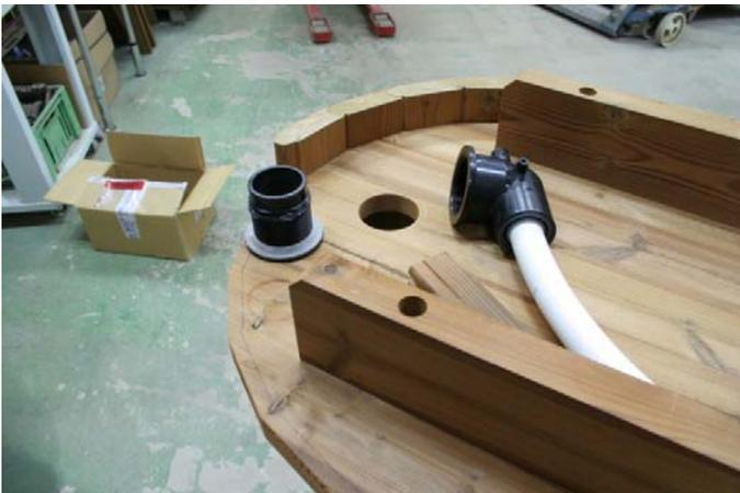
When half the staves are assembled, install the drainage valve. Apply silicone on the threads.
