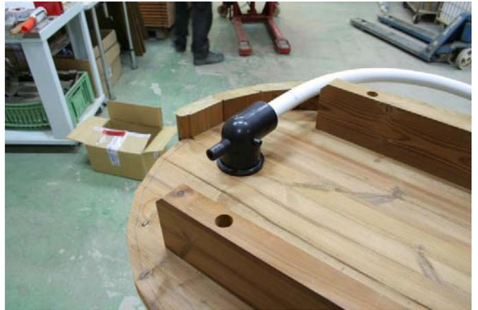
The drainage valve should be turned to the side, or else you will not have access to the drainage hose. The hose will fit in the space between the support leg and stave.
